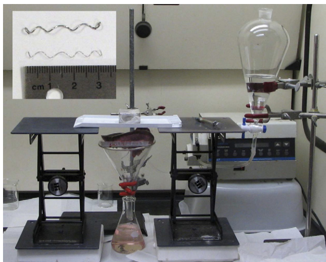
Fig. 1. Photograph of the isolated swine heart ventricle perfusion apparatus used in the in vitro experiments to study IA-MDT.
