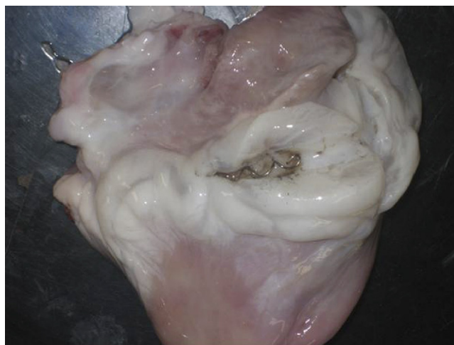
Fig. 5. Photograph of the partially segmented right coronary artery of the isolated swine heart exposing the stent and traces of the magnetite nanoparticles after an IA-MDT experiment. The flow rate was 40 mL/min, the stent wire diameter was 500 \mu\text{m} and the magnetic field strength was 0.125 T.
